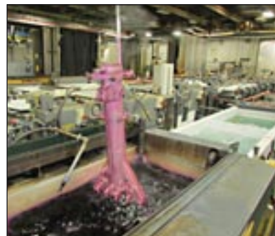
An F-15 outer piston is anodized and sealed with new potassium permanganate sealer at Ogden Air Logistics Complex. AFRL researchers identified and tested this non-chromium sealer as a safer alternative to chromium-based products, and it is now fully incorporated into OO-ALC's coating process. (U.S. Air Force)
